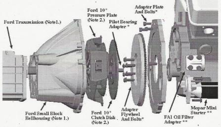
NOTE 1. USE THE FORD SMALL BLOCK BELLHOUSING, THROWOUT BEARING AND LINKAGE (FORK) THAT WERE STOCK TO YOUR TRANSMISSON  $\dot{}$
