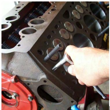
Passengers side hole is partialy covered by the gasket but it will leak if not plugged. There is a water passage on the head that almost lines up with this hole which is why it also needs to be plugged.
