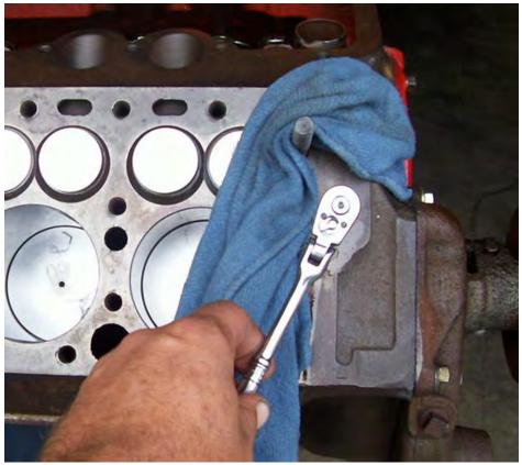
needed. I should be using a tap handle at least or better yet a tap fixture to keep it square and straight.
